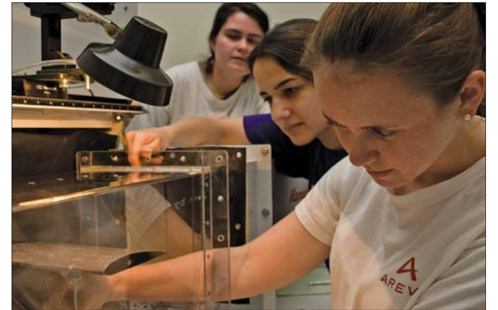
Sweet Briar junior Victoria Nilsson (from left), assistant professor of engineering Dorsa Sanadgol and 2008 graduate Christina Johnson set up a wind tunnel to test the effects of adding electrostatic charge to airfoils.
